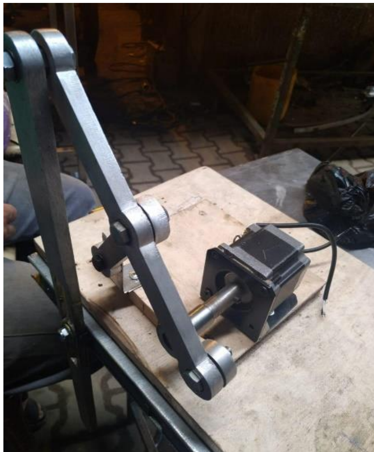
Figure 12: Constructed model (1-DOF) leg mechanism.
