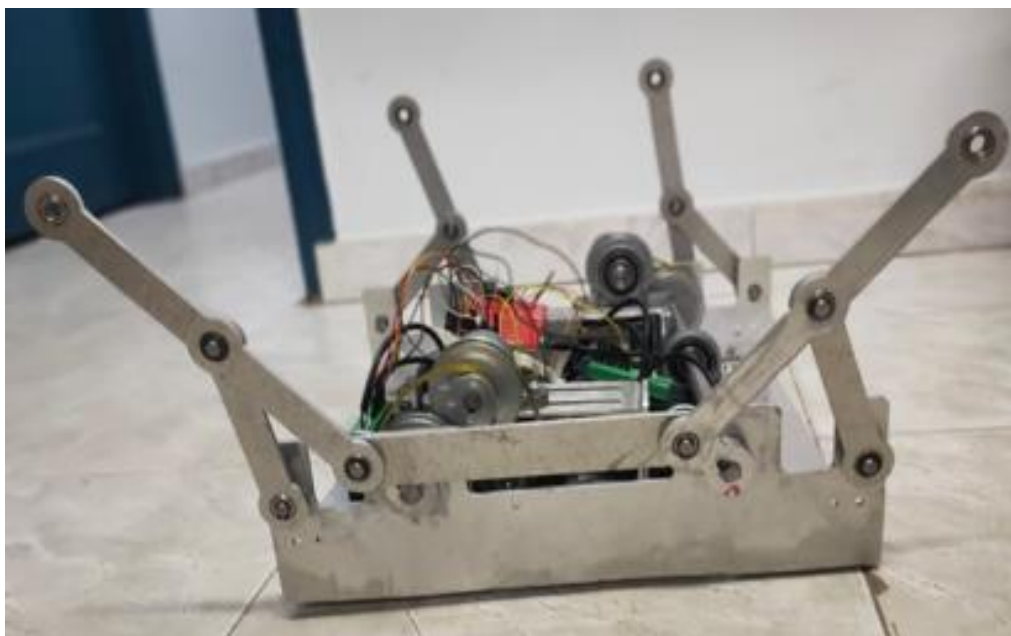
Figure 13: Fully assembled four-legged robotic mechanism.
